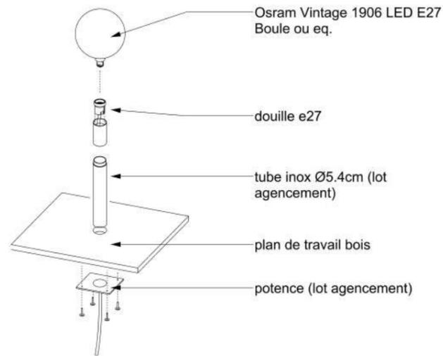
PRINCIPE ASSEMBLAGE FIXATION POTENCE LUMINAIRE
